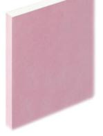
Knauf Fireshield Plasterboard offers improved fire protection when used as part of a full Knauf system. Fireshield Plasterboard can be used in applications that require greater fire protection in systems such as shaftwalls, C stud linings and partitions.
